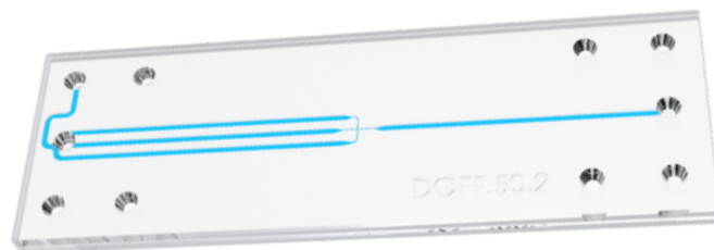
Figure 3: Drawing for 50 \mu\text{m} Top connect Focused Flow Droplet Generator
