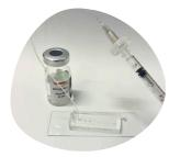
Inject the surface treatment into the channels using a syringe connected to a tubing. Place a filter at the outlet of the syringe to prevent dust from being injected into the channels.
