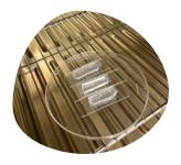
For Fluo-ST3™ treatment, rinse the chip with a fluorinated oil to remove any traces of silanes, then flush the channels with an inert gas.
