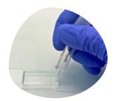
Then flush the channels with an inert gas (e.g. argon, nitrogen) to dry them.
