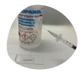
Clean the chip to be treated by injecting isopropanol into the channels using a syringe connected to a tubing. Place a filter at the outlet of the syringe to prevent dust from being injected into the channels.
