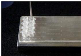
LAMP step 1: Closing chip ports
