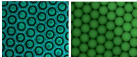
Green light filtered (Ex: 480 nm/ Em: 535 nm) bright field (left) and fluorescence (right) images showing LAMP of target genes (2 ng  $\mu\text{L}^{-1}$  template DNA) within droplet reactors.
